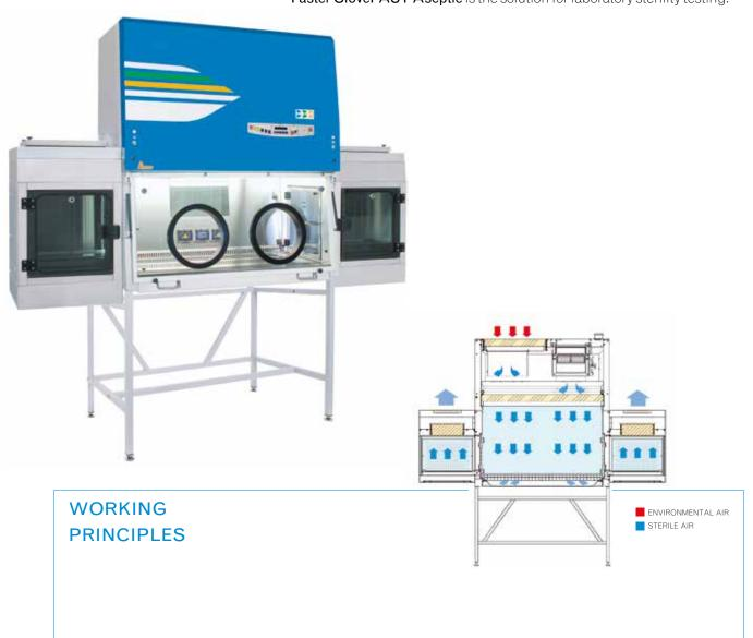
Ambient air is pulled from the H14 HEPA/ULPA filter inlet positioned on top of the isolator and then pressurized downwards towards the work surface prior to be H14 HEPA/ULPA filtered by the main filter. The air is partially re-circulated and partially exhausted via side transfer hatches before being washed again by virtue of a double set of H14 HEPA/ULPA filters fitted inside the hatches.
